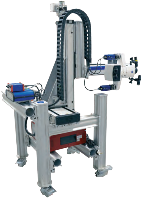
Complete micro-DIC system on moveable cradle
